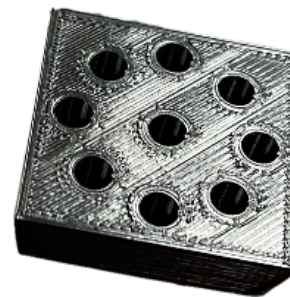
Fig. 7. 3D printed payload (2) - PLA - 20-percent Infill
