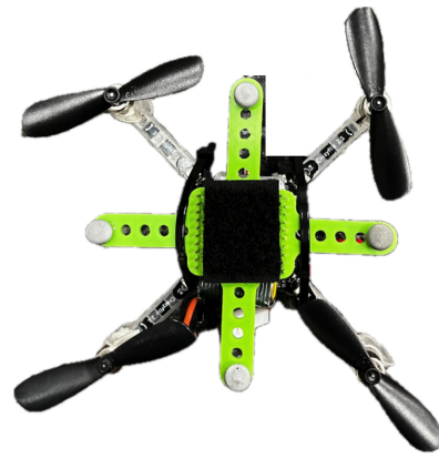
Fig. 5. Mocap Marker Panel (Green, PLA-20-percent Infill)
