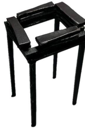
Fig. 6. 3D printed payload (1) - PLA - 20-percent Infill
